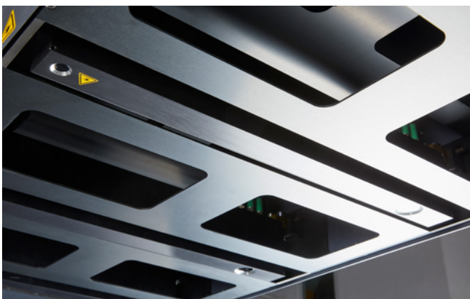
Figure 2: Sensor unit with line laser and camera integrated in the system gantry as the basis for flatness measurement using the laser light section method (Copyright: nokra, now part of KELK)
