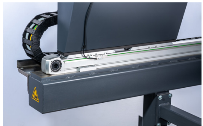
Figure 3: The gantry moves over the sheet metal on precision rails. The servo-controlled linear guide ensures precise measuring operation (Copyright: HIWIN)
