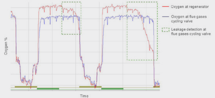
Fig. 16: Oxygen measurements in two locations allows enhanced maintenance operations of the flue gas cycling valve. (Source: Tenova Italmimpianti)
