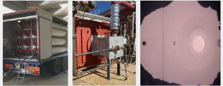
Fig. 12: Setup for the experimental tests of the Tenova TRGX Hydrogen-Ready burner: hydrogen bottles on the truck trailer (left), test furnace (center) and the regenerative burner prototype firing 100 % hydrogen in flameless mode (right). (Source: Tenova Italimpianti)
